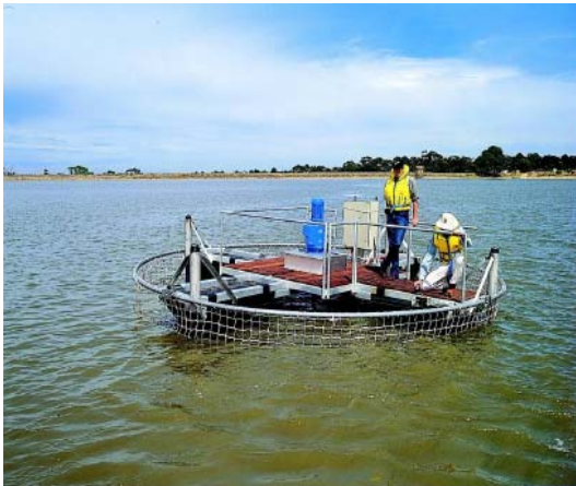
Fig. 19: Mezcladores de superficie. (Foto: gentileza Dr. Michael Burch-CRC for water quality and Treatment-University of Adelaide-Australia)
